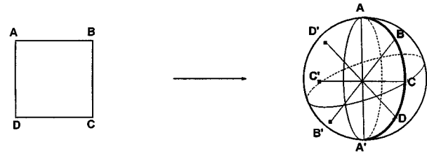
FIG. 4. The disclination-finding algorithm. The directors at the corners of the lattice cube face shown on the left are tracked on the order parameter space sphere shown on the right. The diameters AA' , BB' , CC' , and DD' correspond to the axes of the headless director at the real-space lattice sites A , B , C , and D , respectively.
